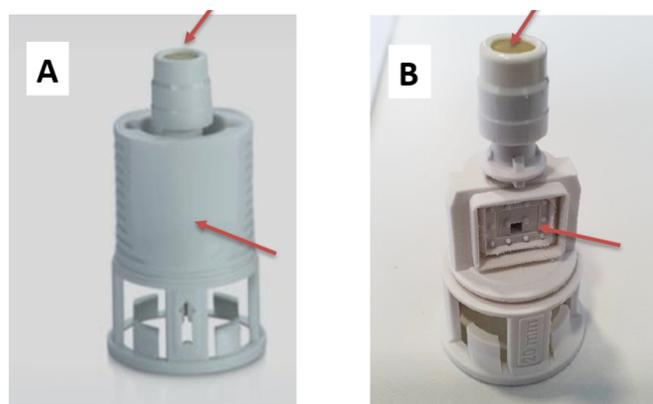
Figure 2. Tested CSTDs with challenged areas. CSTD were either intact vial adaptor (A) or vial adaptor lacking both the sterilizing membrane and activated carbon system (B). The challenged areas sprayed directly with HCoV-OC43 stock solution are indicated by red arrows
