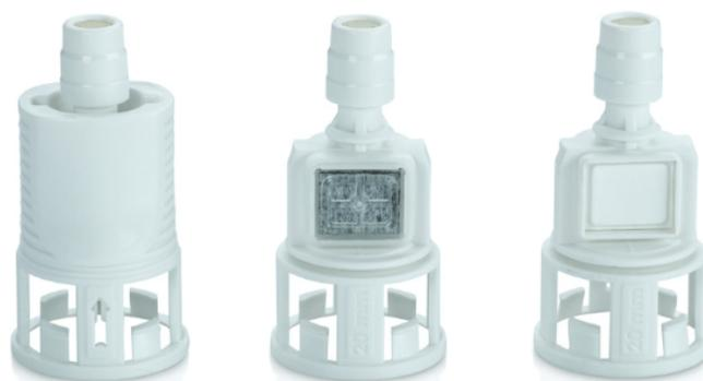
Figure 1. Chemfort CSTD with Toxi-Guard System. Vial adaptor, which firmly connects to any standard vial (left), equipped with the Toxi-Guard system with a 100% activated carbon drug adsorbing matrix (middle) and a 0.2 micron hydrophobic and oleophobic membrane (right), serving together as an effective sterile, particulate, and toxic drug vapor barrier.
