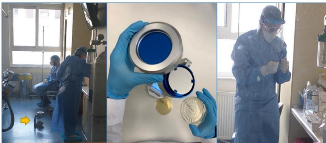
Figure 1: The MAS-100 air sampler and Petri dishes positioning on the room and sampling.
