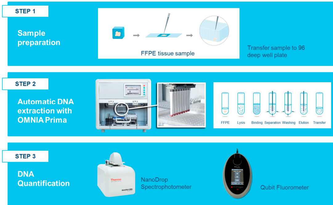
Figure 10. Workflow DNA analysis using the OMNIA Prima automated workstation. Step 1 shows the manual transfer to a well of the processing plate (96 deep-well plate) for each sample. Step 2 represents the fully automatic DNA extraction by the OMNIA Prima workstation. The magnetic tool of the workstation was used to catch the DNA charged beads and to wash and elute the DNA. Step 3 indicates the preliminary evaluation methods used to quantify the nucleic acids before NGS library preparation.
